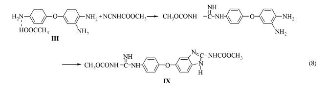
Thus the preparation of methyl 2-benzimidazolyl carbamates **VII** and **VIII** from the corresponding triaminodiphenyl ethers **III** and **IV** requires the application of weak acids, for instance, of acetic acid. But the acid should be used in a large excess to avoid the formation of a considerable amount of a side product **IX** (Scheme 8).
