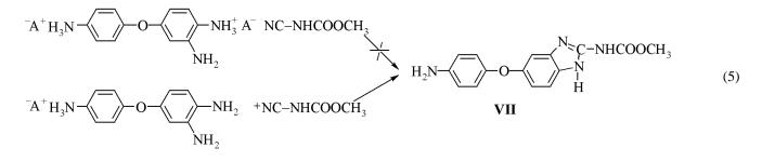
It should be taken into account that the cyclization of triaminodiphenyl ethers **III** and **IV** in the presence of methyl cyanocarbamate occurs with ammonia liberation; the latter can bind the acid necessary for blocking the aniline nitrogen. Therefore it is necessary to add acid into the reaction mixture during the course of the process to maintain the optimum pH.
