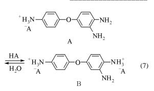
The equilibrium position depends not only on dilution but also on the strength of the acid used for protonation. At the use of a strong acid, e.g., of hydrochloric acid, at equimolar ratio of triaminodiphenyl ether-acid the ethers would exist prevailingly in form A; at the ratio 1:2 the form B would dominate.
