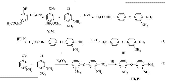
In keeping with Scheme 1 diphenyl ether III is obtained from a solution of 4-acetylamino-3,4-diaminodiphenyl ether I by boiling for 1-2 h in 5% water solution of hydrochloric acid under a nitrogen atmosphere. Along the Scheme 2 were prepared both isomers of triaminodiphenyl ethers **III** and **IV** [3].
